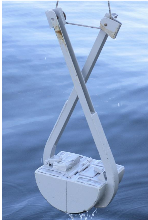
Figure 1.5 A Van Veen grab works like a claw to grab sediment containing macrofauna from the seafloor.
