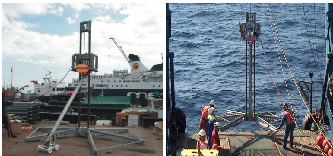
Figure I.7. Left: An example of vibracorer instrument used to sample sediment samples from the seabed; Right: A vibracorer being deployed from a sampling vessel (image sources: GEO Marine Survey Systems, 2011).
