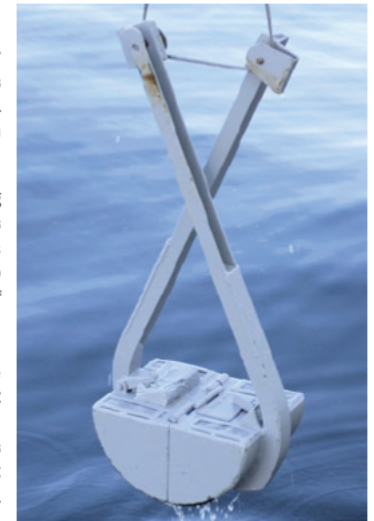
Figure 5 A Van Veen grab works like a claw to grab sediment containing macrofauna from the seafloor.
