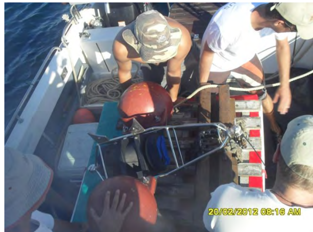
Plate 3: Acoustic Doppler Current Profiler being deployed.
